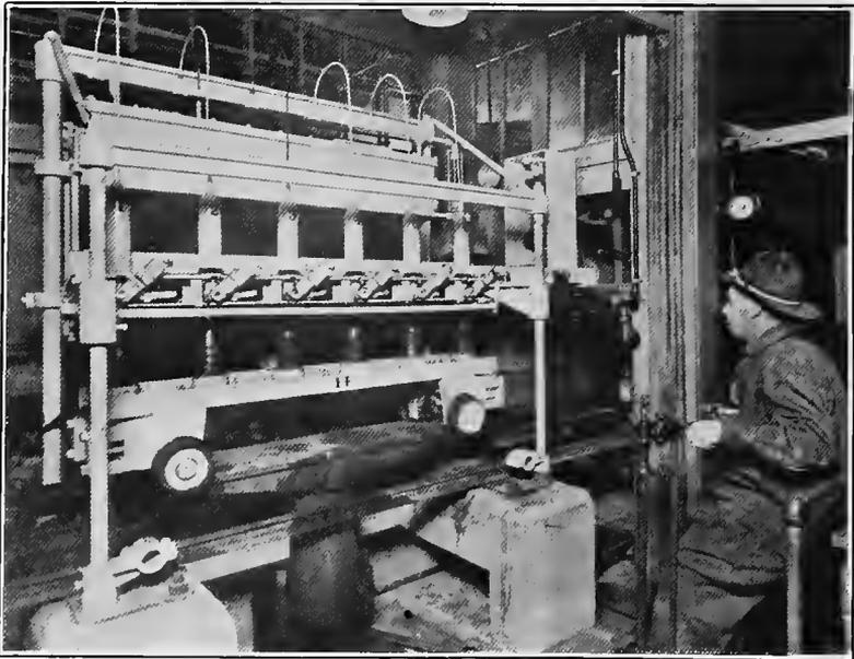
**MACHINE FILLING 75-MILLIMETER SHELL WITH MUSTARD GAS.**
