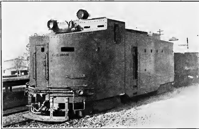
ARMORED MOTOR CAR, OIL-ELECTRIC ENGINE.
