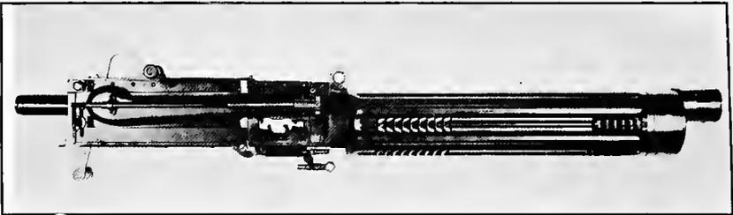
VICKERS AIRCRAFT MACHINE GUN, MODEL 1918, CALIBER .30.
