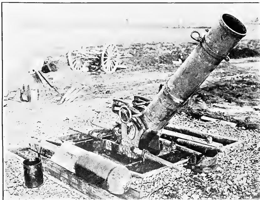
240-MILLIMETER TRENCH MORTAR.
