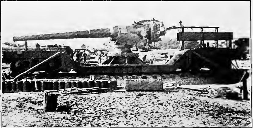
TWO VIEWS OF THE 7-INCH NAVY RIFLE MOUNTED ON A PEDESTAL ON A RAILWAY CAR.
